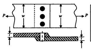
plate width  $w = 200 \, mm$ plate thickness t = 5 mmnumber of rivets n = 3rivet diameter  $d_r = 10 \, mm$ rivet hole diameter  $d_4 = 11 mm$ allowable tensile stress of plate  $\sigma_p = 200 MPa$ allowable bearing stress of rivet  $\sigma_c = 150 MPa$
